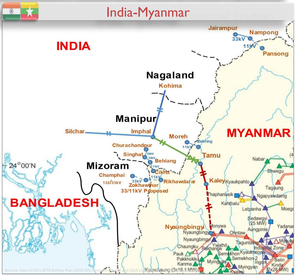
Imphal (India) - Tamu (Myanmar) AC line along with 1x500 MW HVDC back-to-back
