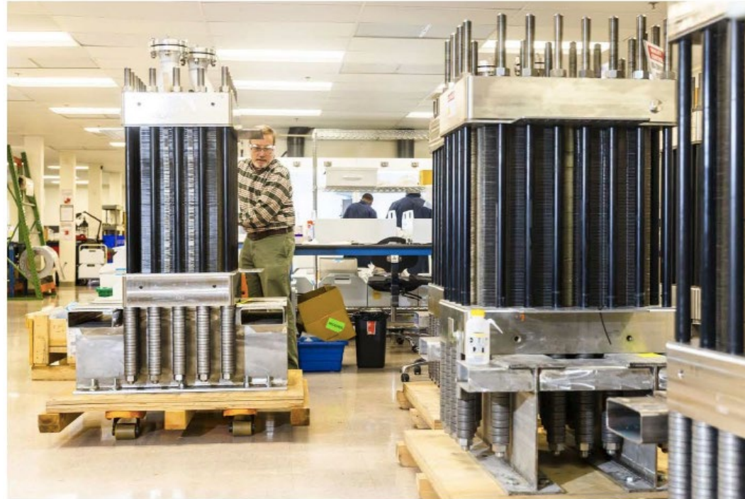
All electrolyzer stacks contain oppositely charged electrodes — cathodes and anodes — as well as an electrolyte. The Plug Power electrolyzer stacks shown here use a technology called “proton exchange membrane” or PEM, which features a solid electrolyte. Photographer: Adam Glanzman/Bloomberg
