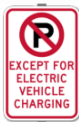
FIGURE 5-12: RECOMMENDED SIGNAGE FOR EV CHARGING
