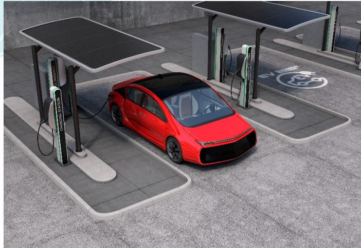
FIGURE 3-37: CHARGING STATION WITH SPACES LEFT BETWEEN VEHICLES
