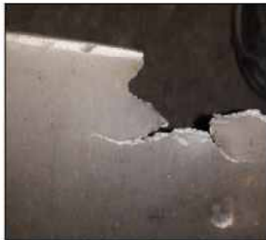
Figure 31: PA fan blade failure due to stalling
