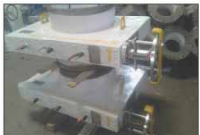
Figure-41b: Installed BMW Variable orifice
