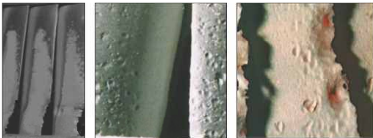
Figure-22: a. Exfoliation of turbine blades, b. Pitting, c. Damage to nozzles
