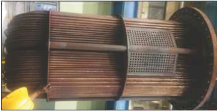
Figure 14: HP heater tube bundle
