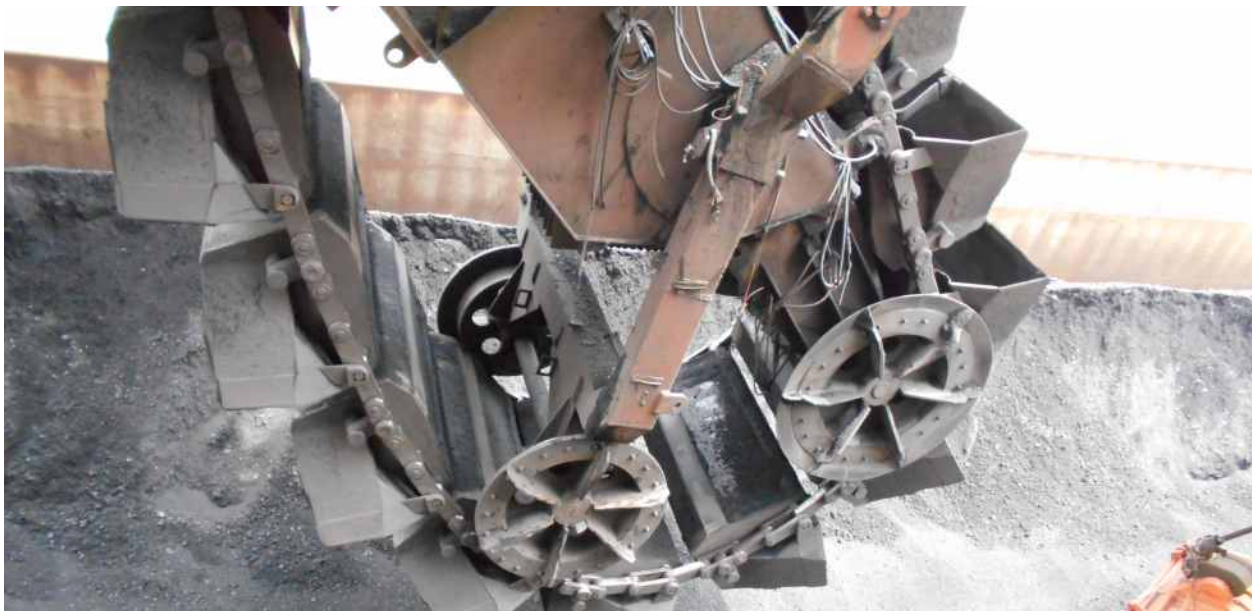
USAID PACE-D TA Program Study Tour to U.S. in July 2013: Coal Reclaimer at AEP Amos.
