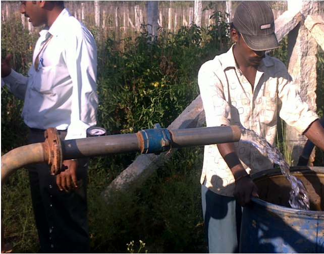
Monitoring of water discharge from energy efficient pump set at the pilot site.
