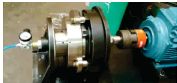
Initial test of novel scroll expander for organic Rankine cycle
