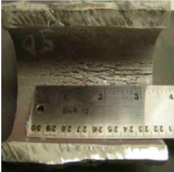
Figure 5-3: Corrosion Fatigue Cutaway
