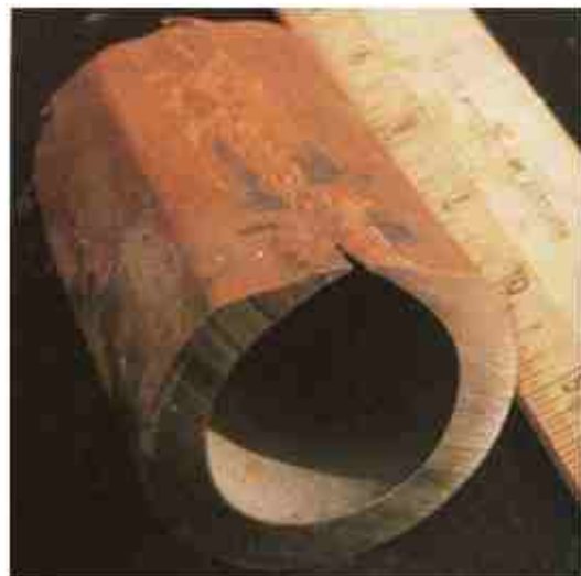
Figure 9-49: Coal Particle Abrasion
