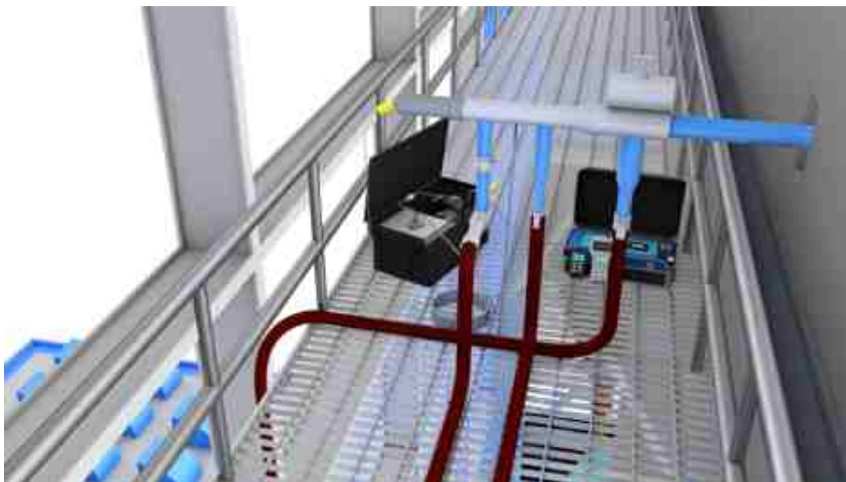
Figure 6-16: High Velocity Thermocouple (HVT) – with Monorail System
