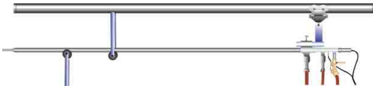
Figure 6-56: Monorail Concept For "User Friendly" HVT Measurement
