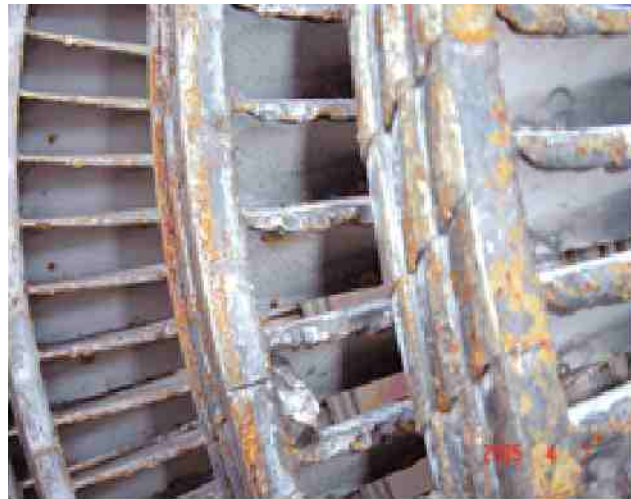
Figure 5-6: Catastrophic Turbine Failure (Sodium Salts)
