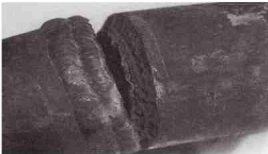
Figure 9-41: Dissimilar Metal Weld Failure
