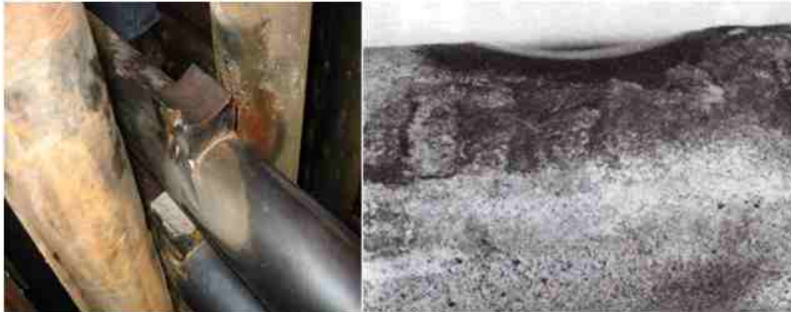
Figure 9-47: Rubbing and Fretting
