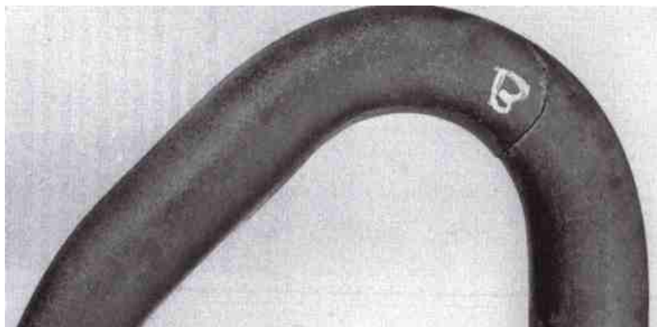
Figure 9-50: Low Temperature Creep
