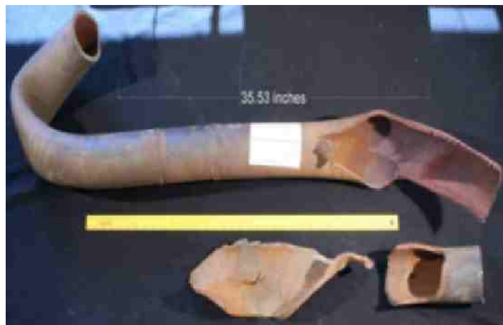
Figure 5-2 : Corrosion Fatigue Boiler Tube Failures
