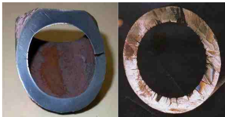
Figure 9-36: Stress Corrosion Cracking
