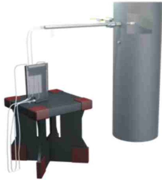
Figure 6-42: Dirty Airflow Sampling
