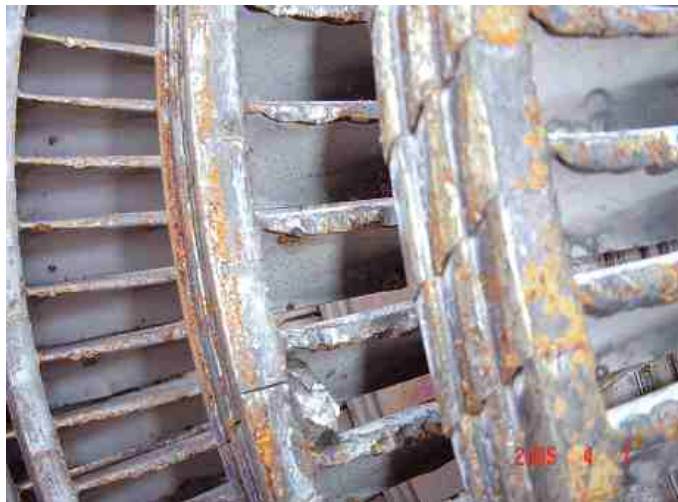
Fig. 5-5: Catastrophic SCC Turbine Failure
