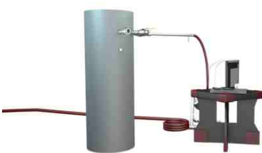
Figure 6-43: Isokinetic Coal Sampling (via Modified ASME sampler)
