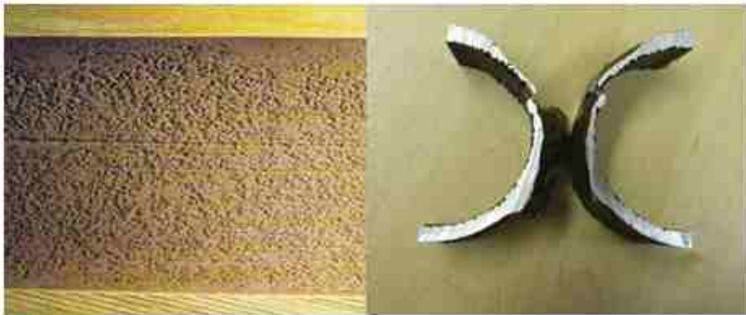
Figure 9-48: Chemical Cleaning Damage
