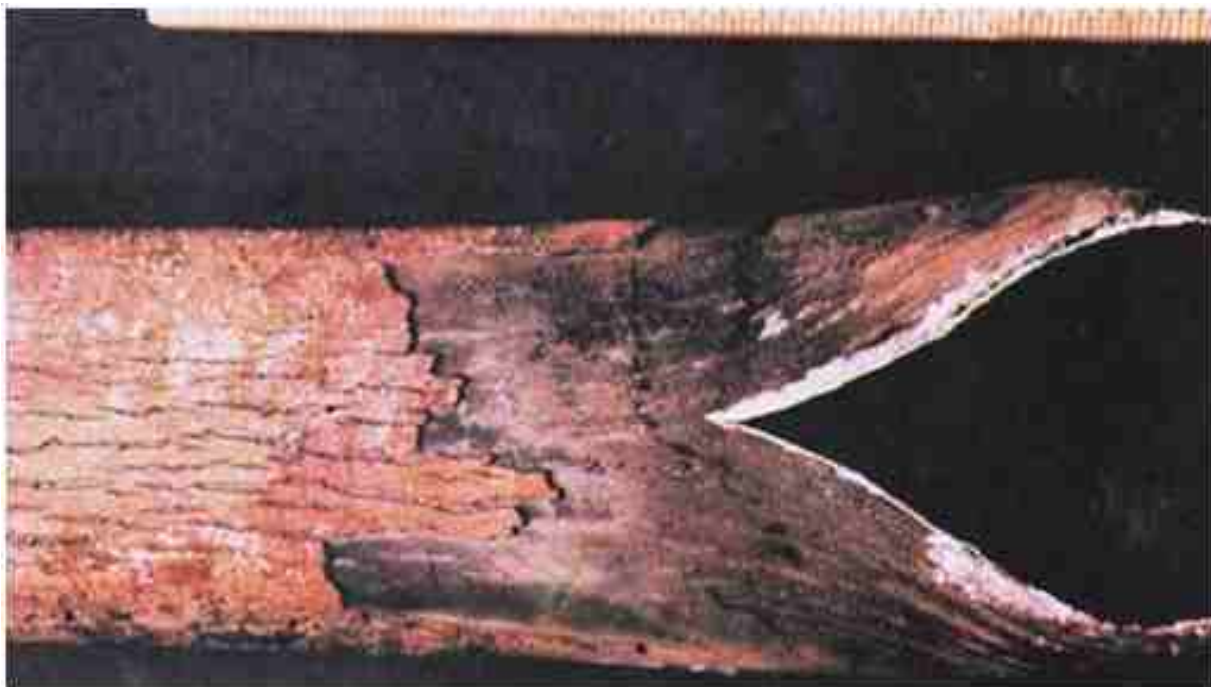
Figure 9-39: Long-Term Overheating and Creep Fatigue
