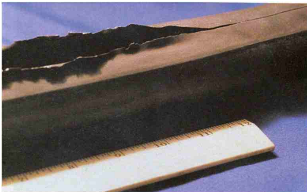
Figure 9-31: Soot Blower Erosion
